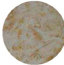
A contaminated filter paper, stained with clay, will deliver erroneous results and over-estimate the moisture content.
